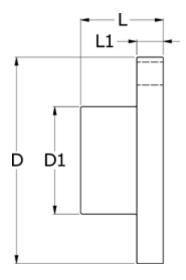
$\begin{array}{lll} D & = 125 \\ D1 & = 65 \\ L & = 50 \\ L1 & = 16 \\ Max \ bore & = 40 \\ Torque \ (N \ m) = 350 \end{array}$
